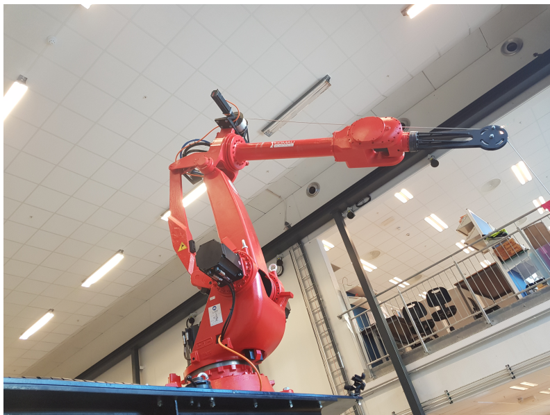
Figure 2.4: Photo of the Comau Smart 5 NJ 110-3.0
