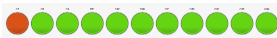
Figure 5.18: Indicators that corresponds to a fault in bearing one according to table 4.8
