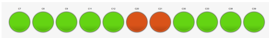
Figure 5.15: Indicators that corresponds to a fault in bearing one according to table 4.8
