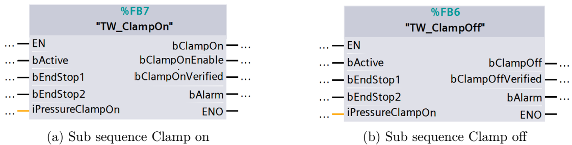
Figure 6.13: Sub sequences block in FBD for Clamp on and off sub sequences
