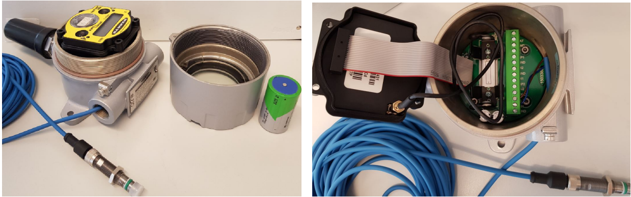
(a) Sensor node, battery and proximity sensor
