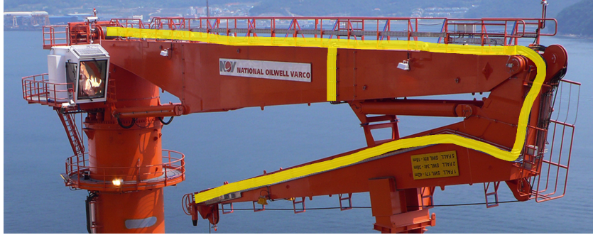
Figure 2.5: Typical piping on offshore crane (yellow marked) [4]
