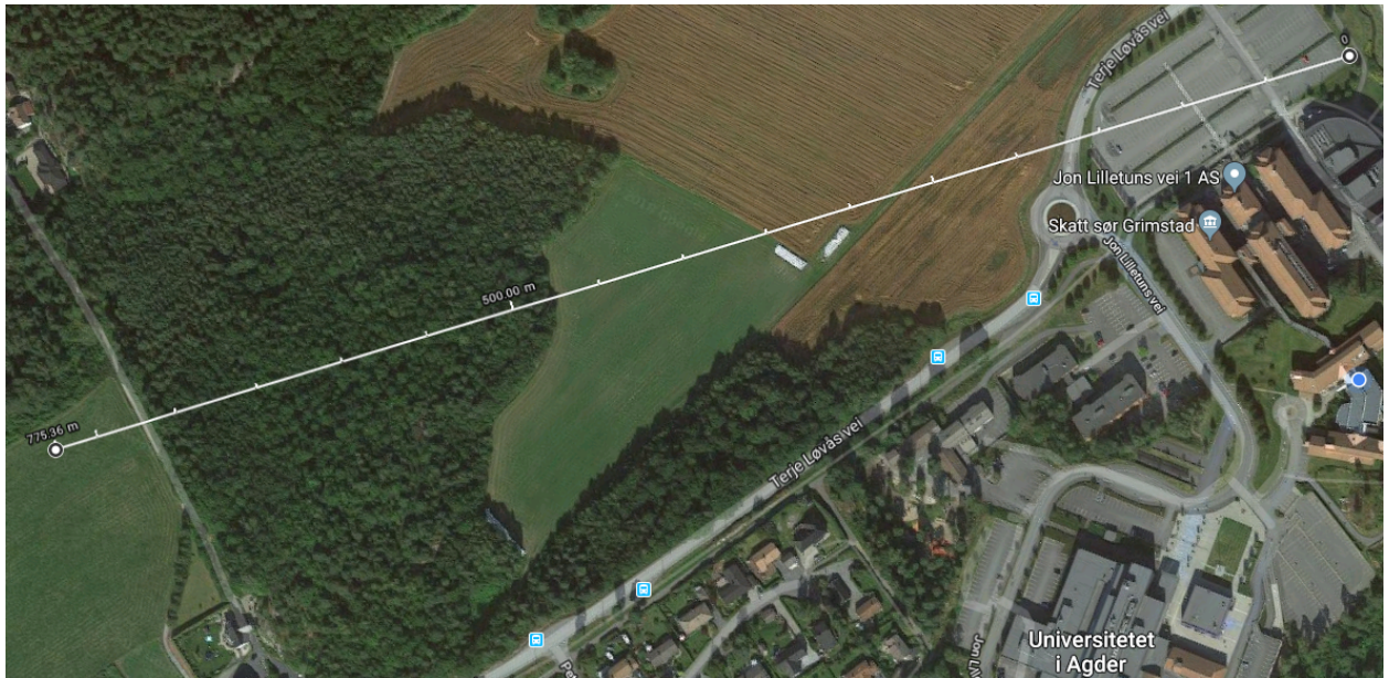
Figure 4.48: nRF52840 range test with 8dBm transmission power and non-coded transmissions
