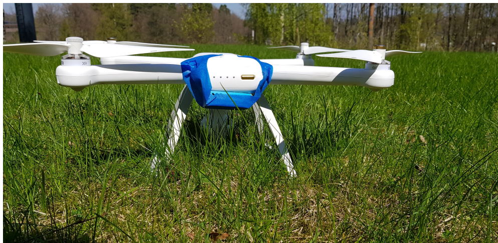
Figure 4.25: Drone with a sensor node placed on the bottom side
