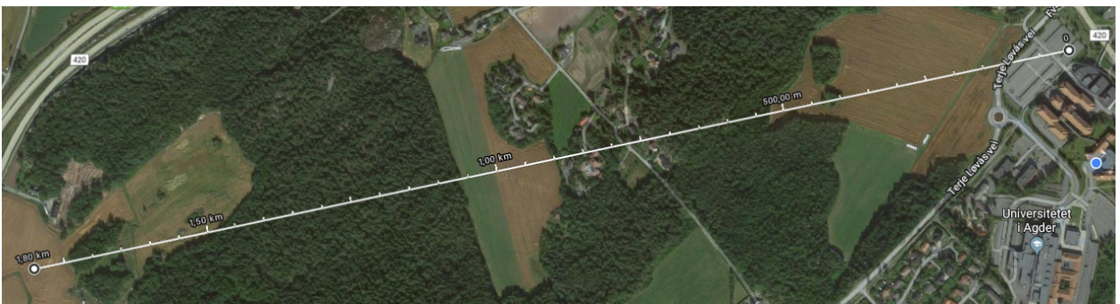
Figure 4.47: nRF52840 range test with 8dBm transmission power and coded transmissions
