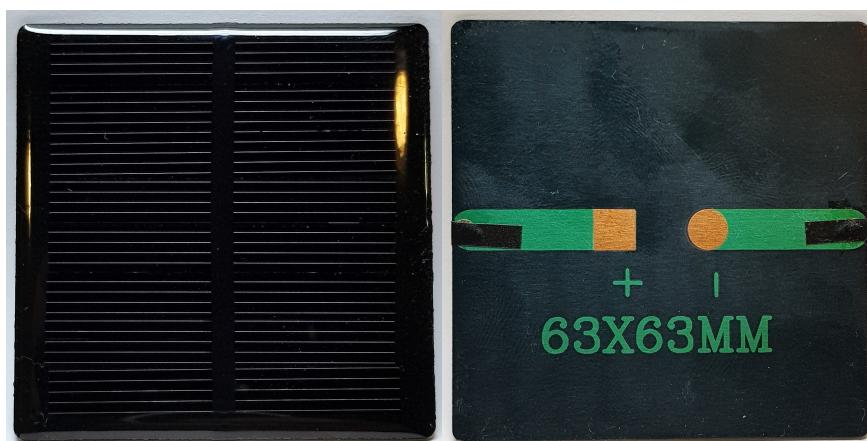
Figure 3.3: Front and back of the 0.36W solar panel
