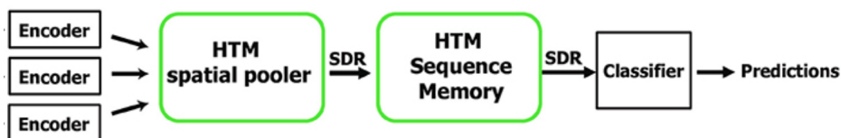
Figure 3.1: Diagram of the HTM architecture [23]. HTM Sequence Memory is synonymous with Temporal Memory in this case, and the Classifier decodes the SDR into a normal representation.
