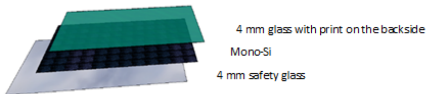
Figure 5.2: Structure of the green printed panel from ISSOL
