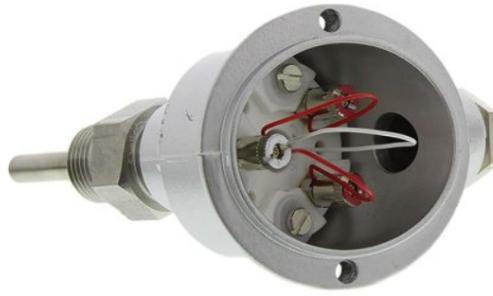
Figure C.16: PT-100 element as mounted on the inlet[74]
