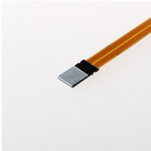
Figure C.18: GreenTeg Flux sensor[76]
