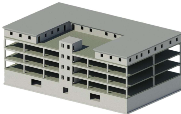
Figure 6.3 Hollow core elements added to the model.
