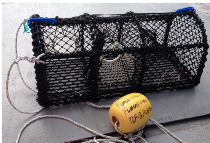
Fig. 2. The modified two-chambered 12 kg parlour trap (dimensions: 35 cm H x 66 cm W x 40 cm D) with two entrances and modifications to reduce ghost fishing. The frame is made of steel and covered with a synthetic net.
