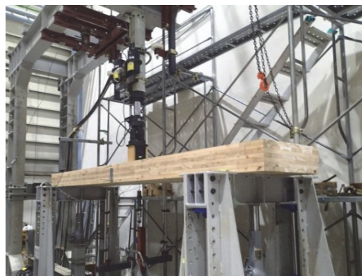
Fig. 2 Repeated loading test of CLT slabs
