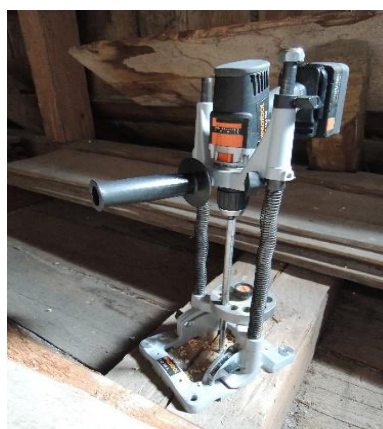
Fig. 7 Special stand to fix the drill with the bit and its fixation to the element
