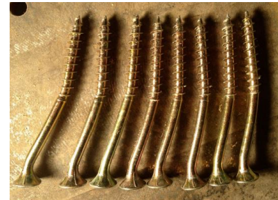
Fig. 15 Ductility due to the formation of 2 plastic hinging on the stem of the screws [9]
