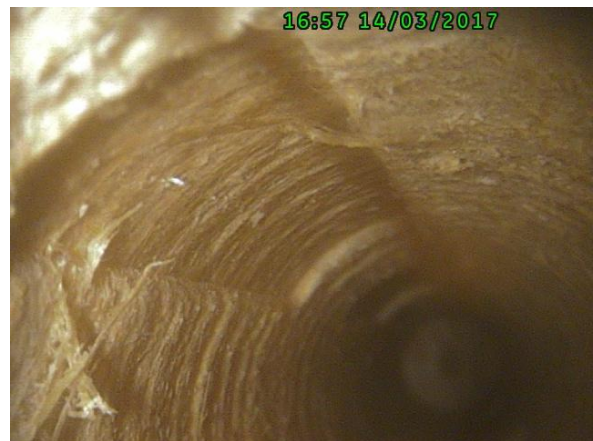
Fig. 8 Detail of the measuring part of the device before insertion in the borehole, diameter of 12 mm Fig. 9 Prints of the jaws in borehole no. 12
