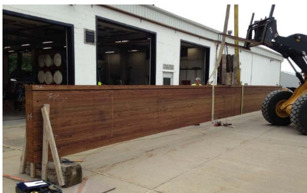
Fig. 11 Girder with weight at midspan during stiffness testing
