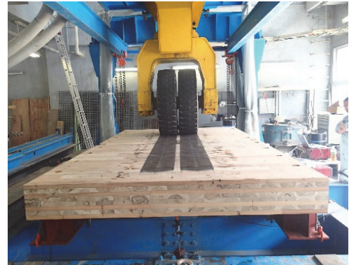
Fig. 4 State of dynamic wheel load test
