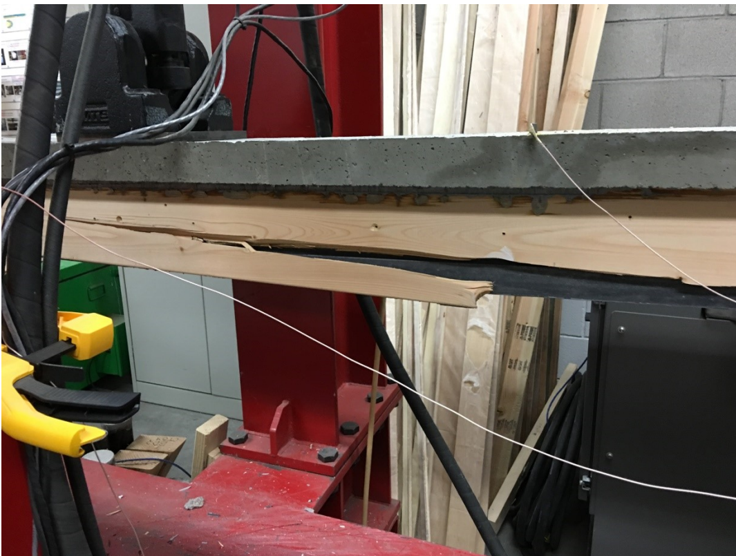
Fig. 5 Failure of the timber in tension and delamination of the timber-steel bonding (S-LTC specimen BM4 shown)
