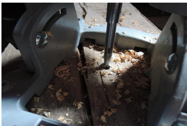
Fig. 6 Detail of the milling bit for the preparation of drilling, diameter of 12 mm
