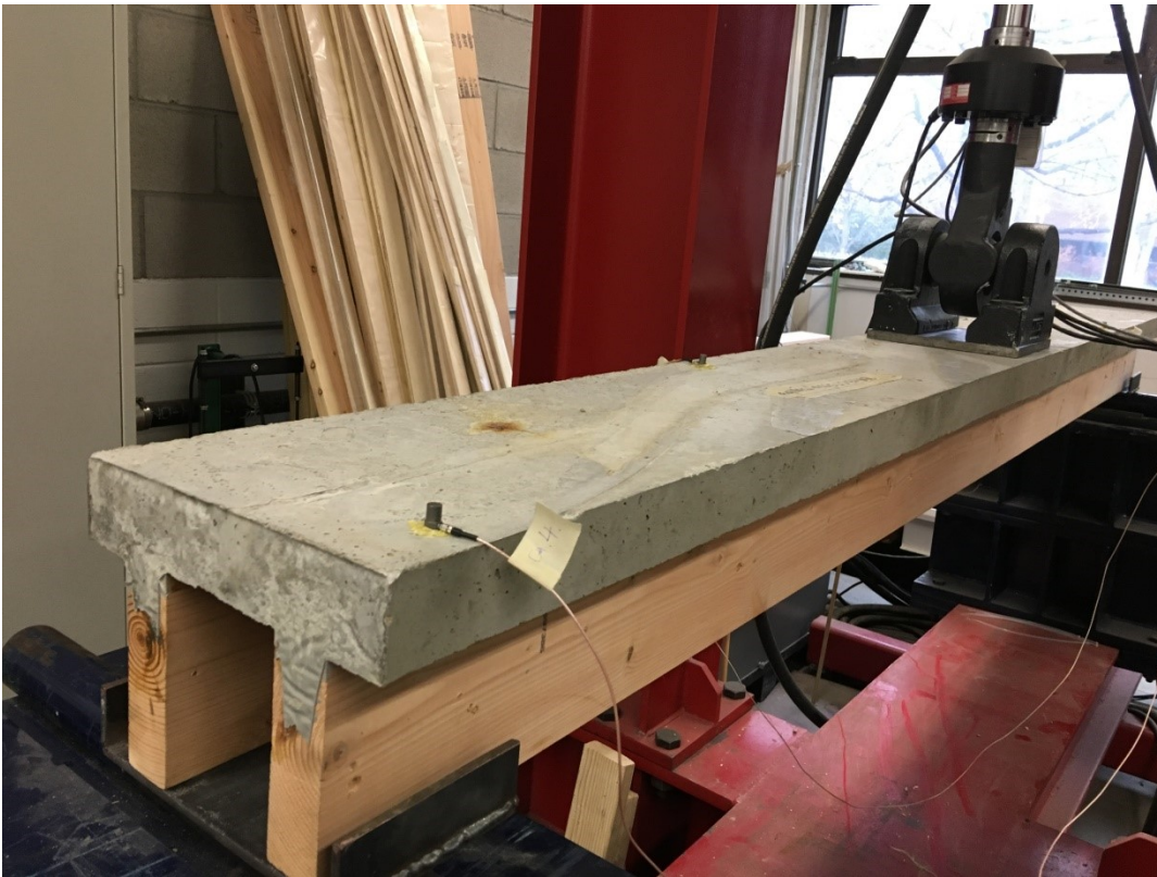
Fig. 1 Typical test setup of an LTC specimen (BM3 shown)
