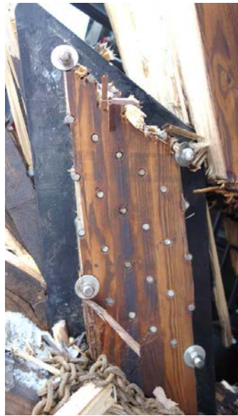
Figure 4 Example of group tear failure (left) and row shear failure (upper) on Perkolo Bridge
