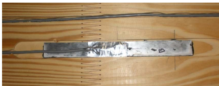
Fig. 8 Shim gage configuration for measuring strains
