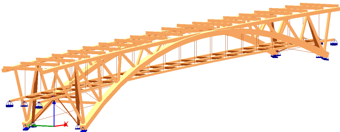
Figure 4 Computation model in Focus Konstruksjon used for analysis and design
