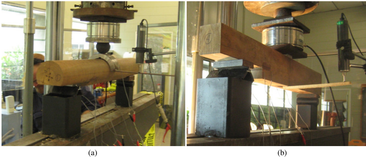
Fig. 4 Experimental test setup (a) Round timber member (b) Rectangular timber member
