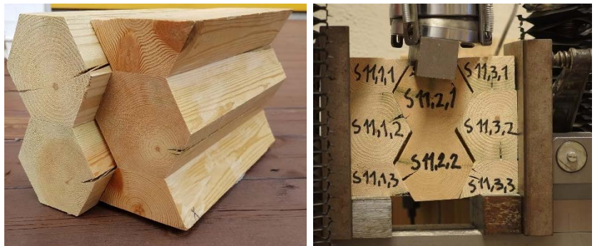
Figure 16 By using hexagonal shapes for laminated timber decks, shear forces may be transferred also by pressure instead of friction only
