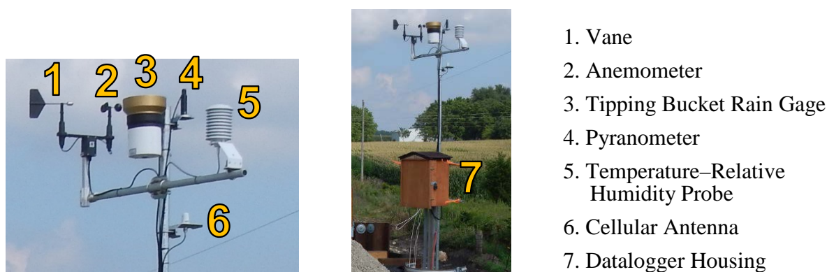
Fig. 5 Ambient weather condition sensors and datalogger housing
