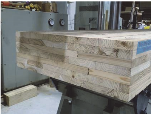
Fig. 1 Laminate composition of CLT slab
