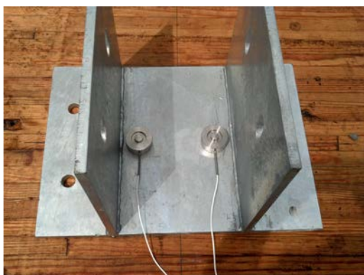
Fig. 10 Welded plate bearing assembly with mounted load cells
