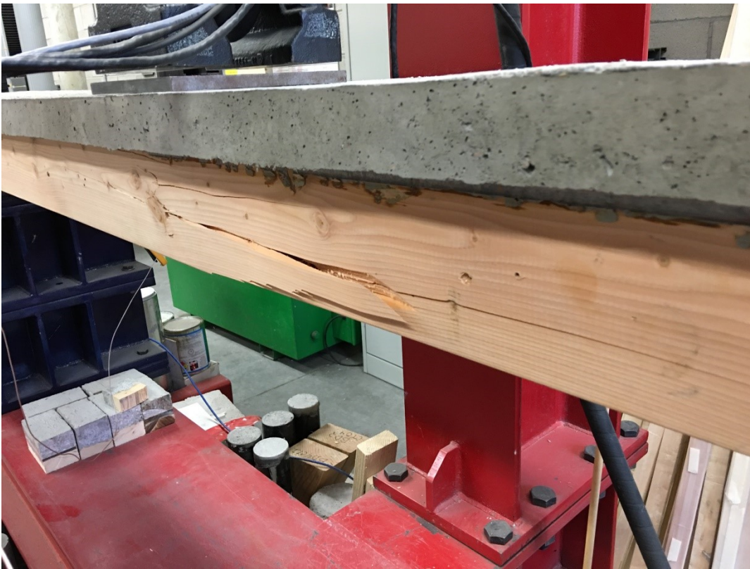
Fig. 4 Failure of the timber in tension (LTC specimen BM3 shown)
