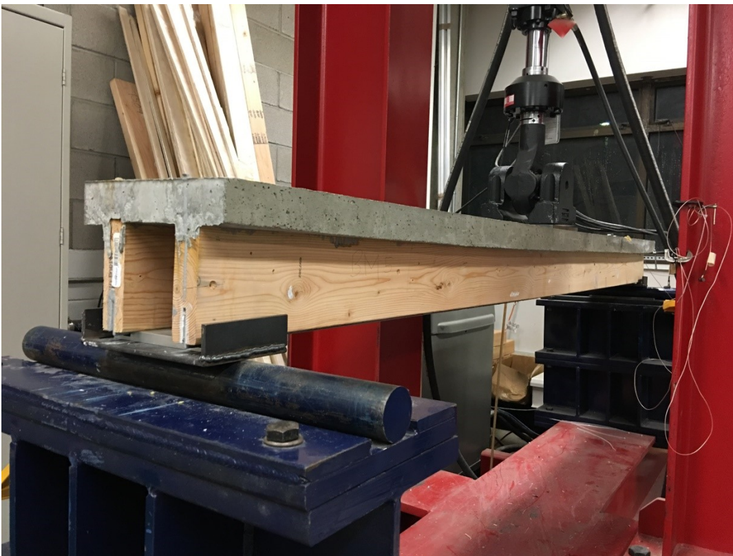
Fig. 2 Typical test setup of an S-LTC specimen (BM5 shown)
