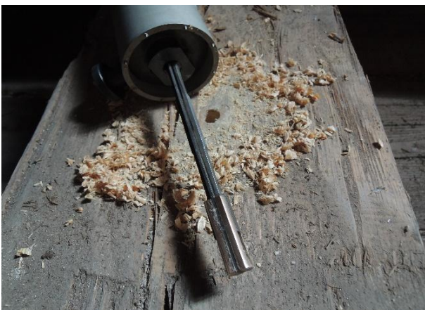
Fig. 8 Detail of the measuring part of the device before insertion in the borehole, diameter of 12 mm Fig. 9 Prints of the jaws in borehole no. 12
