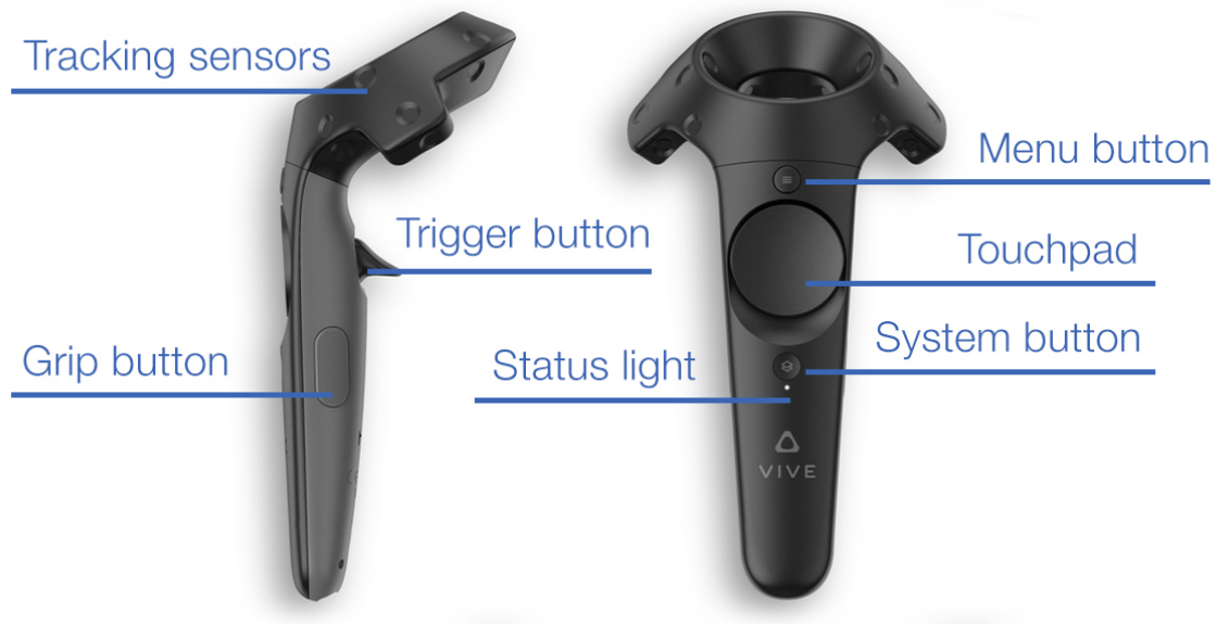
Figure 2.11: The HTC Vive controllers and button names. Adapted from HTC Vive Image Gallery [52]
