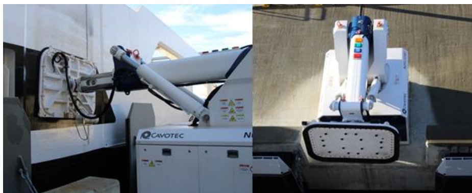
Figure 6-10: The mooring system which is used in MS Ampere, and is expected to be used in the UWS. Photo is taken by Tobias Einberger.
