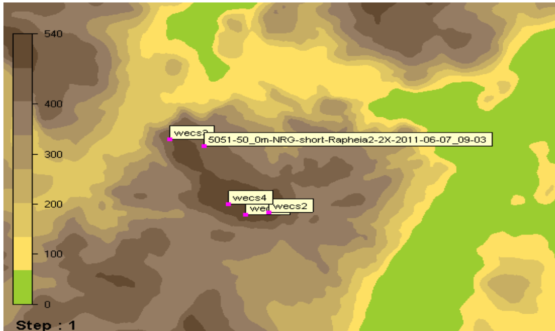
Figure 4.4. Depicts the positioning of wind turbines in the park layout. The elevation level is represented by the color coding with different shades i.e. dark brown shade shows the highest elevation level with 540m.
