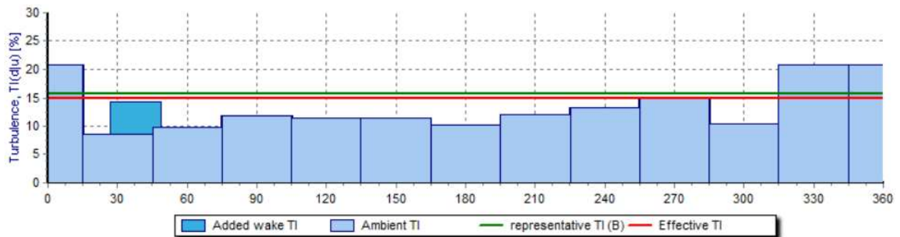
Figure 4.10. Added wake TI is within IEC61400-1 (ed.3) limit, whereas ambient TI exceeds the limit.
