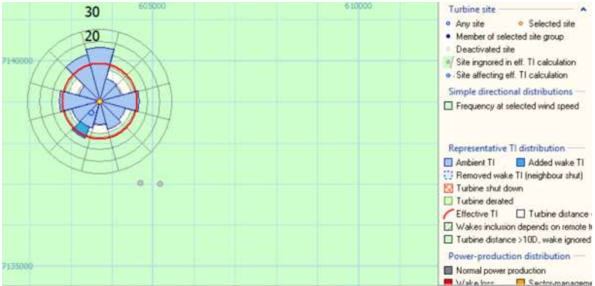
Figure 4.14. The effective turbulence in dependence of wind direction. The ambient turbulence is higher due to the different wind directions within wind farm.
