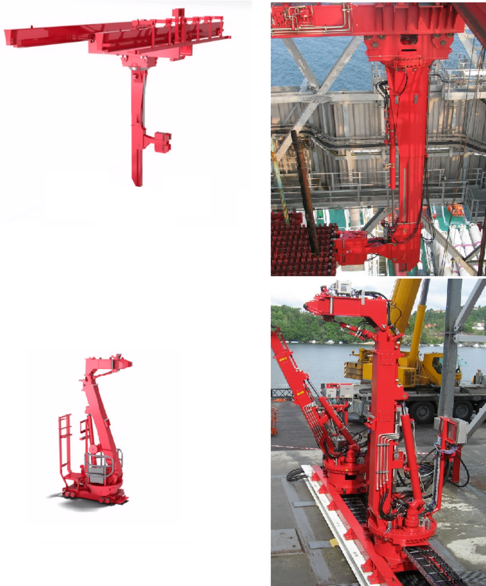
Figure 1.1: Bridge crane and lower guiding arm [9]
