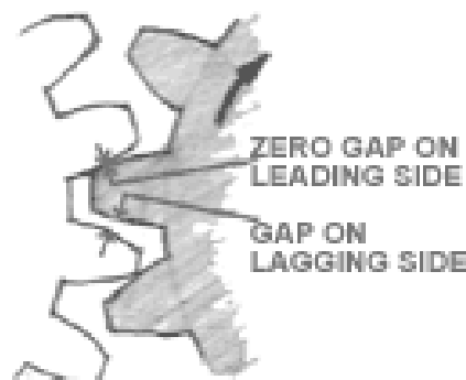
Figure 5-1 Backlash Gap Relative to Driving Direction [56]
