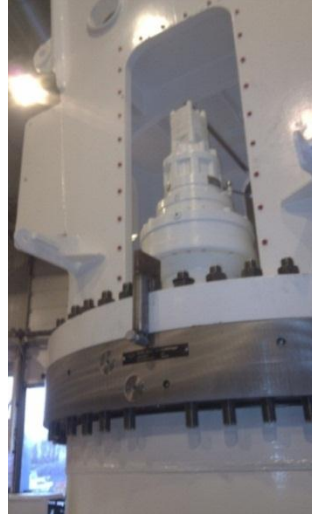
Figure 4-6 Hydraulic Motor Fixed on a Slewing Gear
