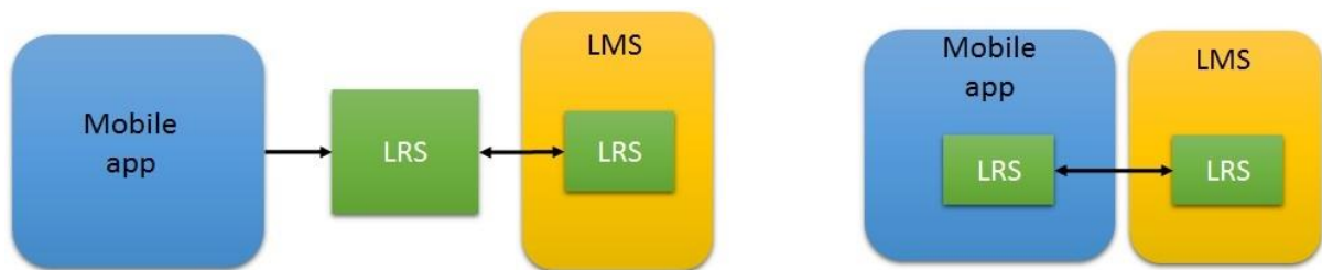
Figure 12 Mobile learning application scenario with internal and external LRS
