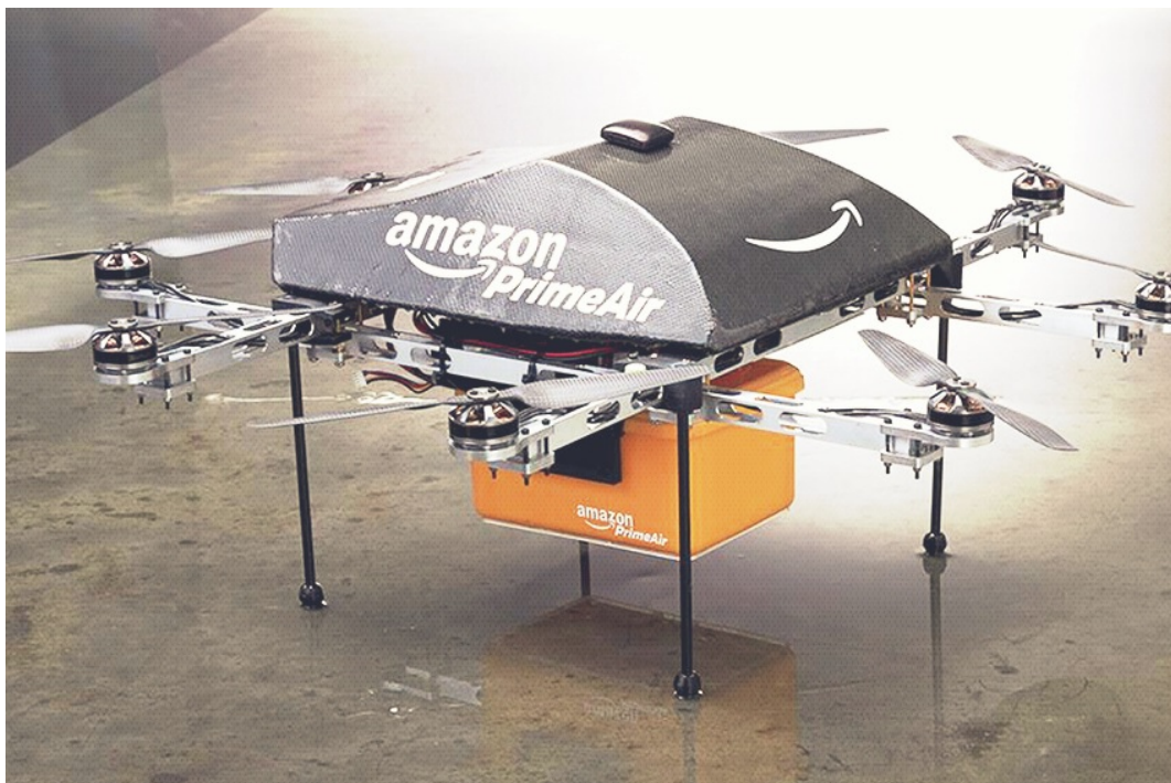
Figure E.1: Example of multirotor UAV design by Amazon for transport and delivery of parcels.
