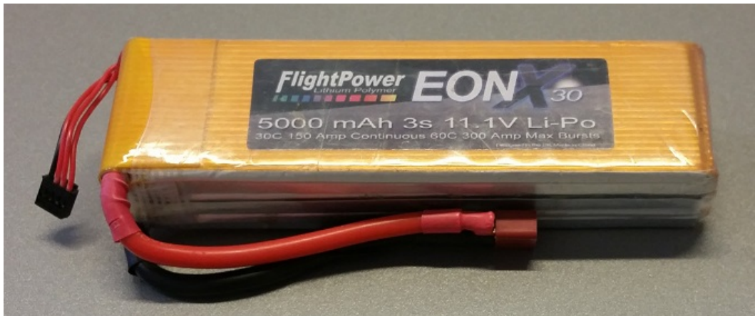
Figure E.7: Battery used in the design validation tests.
