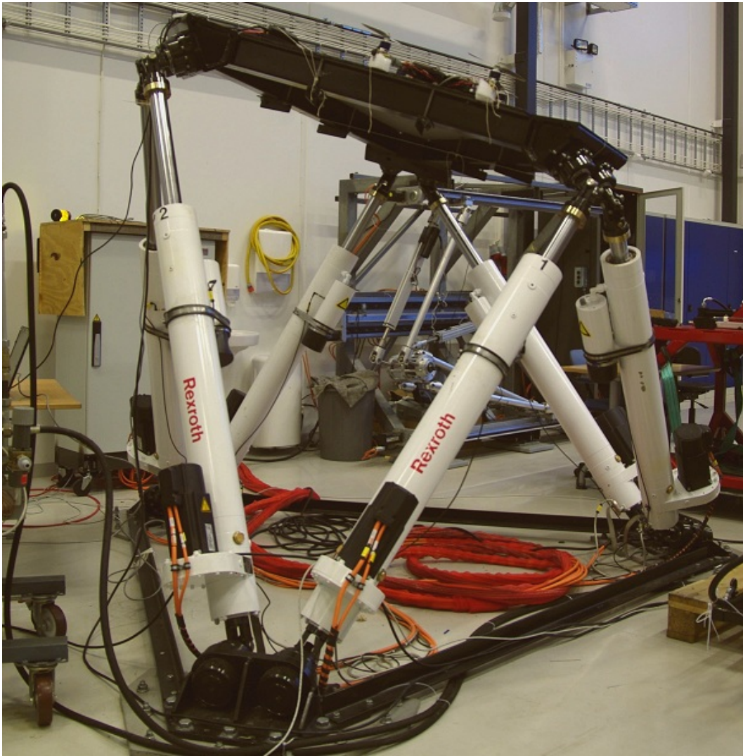
Figure A.4: Stewart Platform used for IMU calibration experiments.
