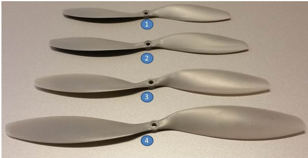
Figure E.6: Four different propellers used in the design optimization and validation tests.
