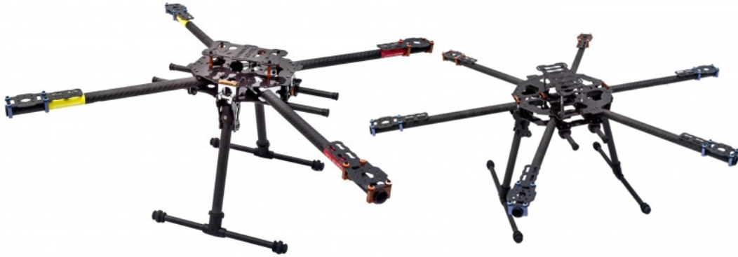
Figure D.1: Examples of two different multirotors used in the design optimization process, a quadrotor and a hexarotor.
