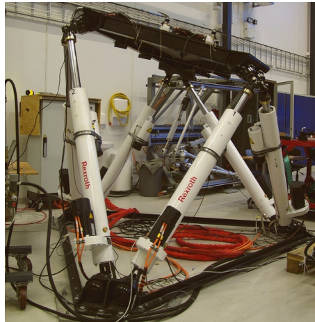
Figure B.7: Stewart platform used for testing
