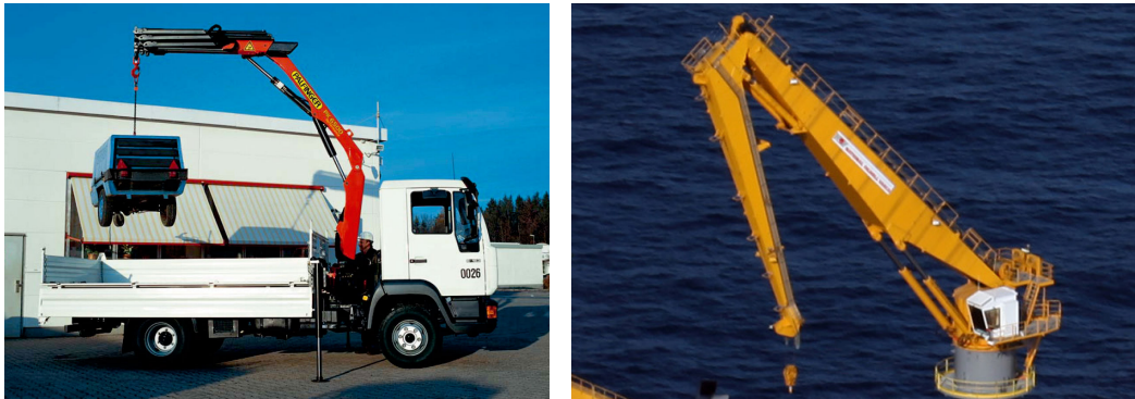
Figure 1.1: Examples of knuckle boom cranes. To the left is shown a mobile loader crane (Direct industry, 2016) and to the right an offshore knuckle boom crane (NOV, 2014).
