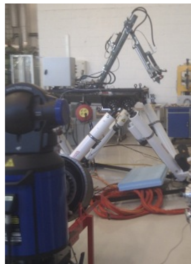
Fig. 1. Experimental setup showing Stewart platform, redundant hydraulic crane and laser tracker for measuring the tool point location.
