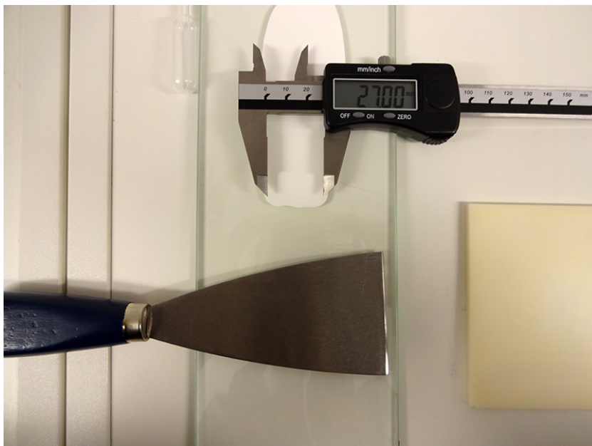
Figure A.14: Measure every sample you cut and shape, so that you are able to track any changes further on in the process, e.g. after sintering.
