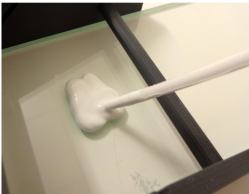
Figure A.8: Do not apply the slurry on to the plate in this manner. You are bound to get bubbles, which you do not want.
