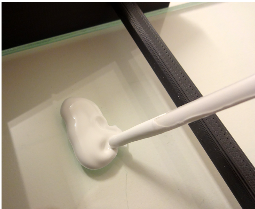
Figure A.9: By keeping the pipet a bit above the slurry, you will reduce the chance of blowing air into it.
