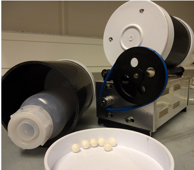
Figure 3.5: Ball-milling equipment and setup.
