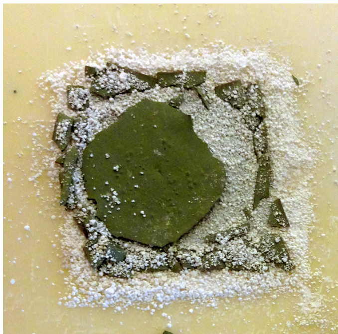
Figure 4.8: Final co-cast anode and electrolyte substrate, sintered at 1300°C. Unsuccessful result.
