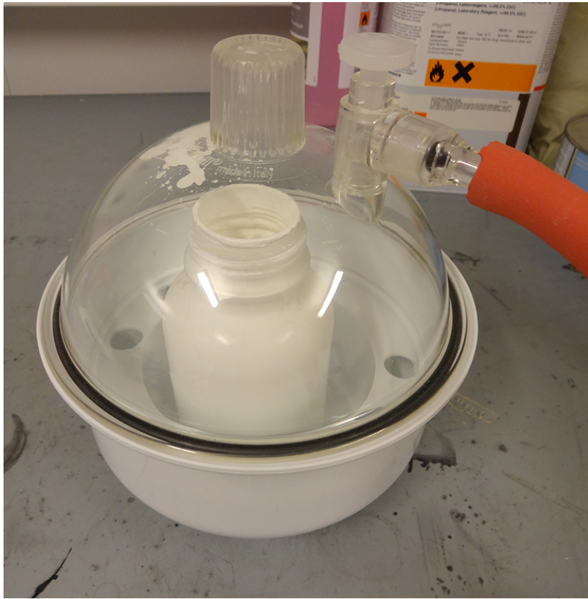
Figure 3.6: Small laboratory vacuum chamber.
