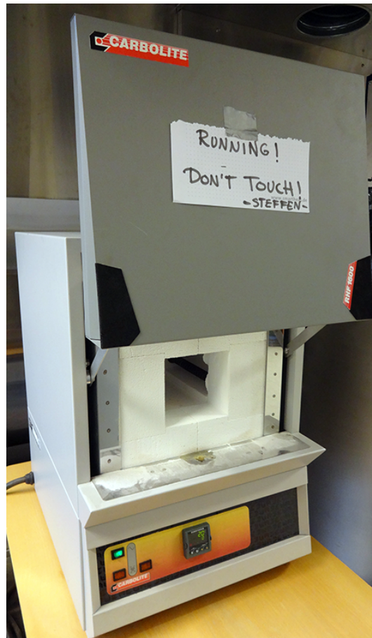
Figure 3.13: Sintering furnace, Carbolite, model RHF 16/3.
