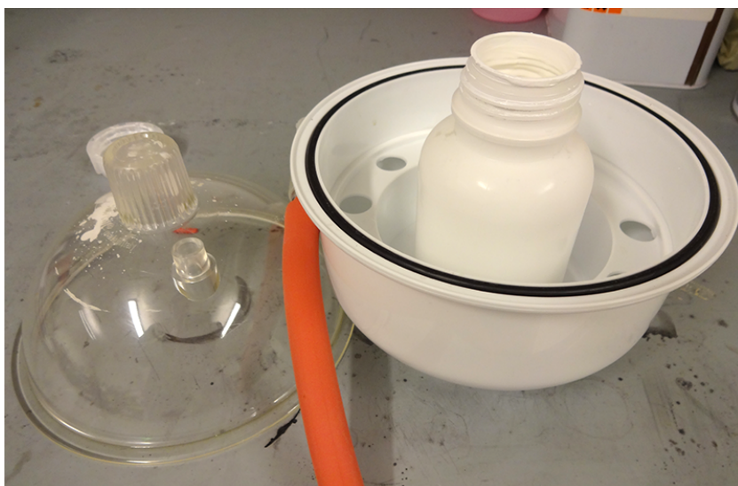
Figure A.1: Vacuum chamber driven by a small water pump connected to and driven by a regular water tap.
