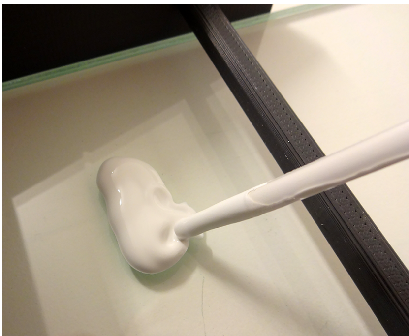
Figure 3.9: By keeping the pipet a bit above the slurry will reduce the chance of blowing air into it.
