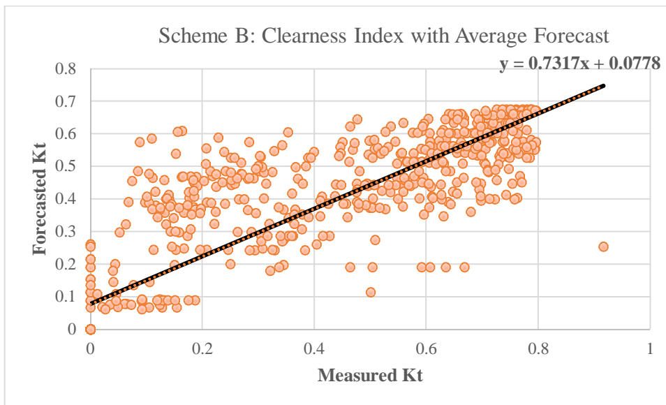
Figure 4.14. Forecasted Clearness Index vs. Measured Clearness Index for the Month-May, 2012 under Average Forecasting Scheme
