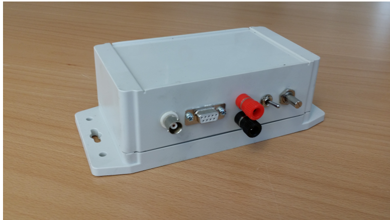
FIGURE 3.10: The connection box used at the generator Suldal 1
