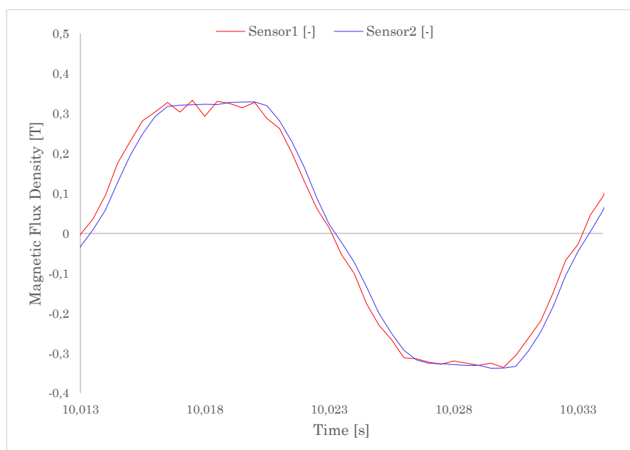
FIGURE 5.2: Close-up of the flux density for one pole-pair at Svante with a magnetizing current of 15 A.
