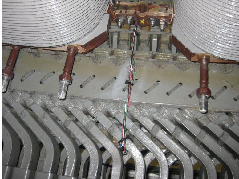
FIGURE 4.7: Cable routing of the lower cables
