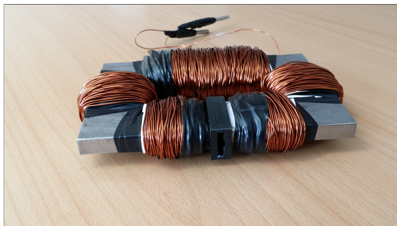
FIGURE 3.4: Picture of the final electromagnet with plastic insert in the air gap
