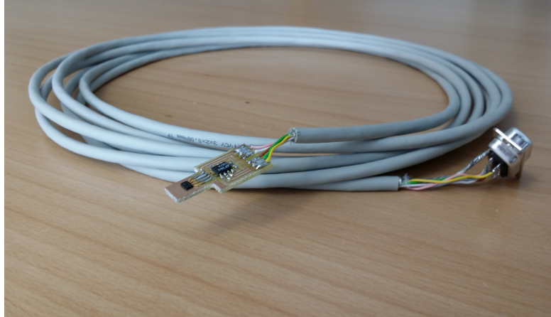
FIGURE 3.8: Complete Hall-sensor with amplifier
