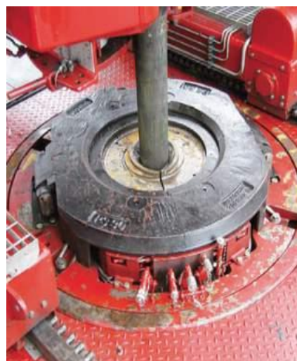
Bilde 3: Hydraulic operated Power Slips (AkerSolutions, 2014b)
