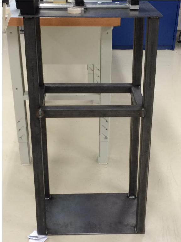
Figure 3.14: The tower structure for the wind turbine
