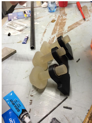
Figure 3.16: The finished print of the bevel gears in housing
