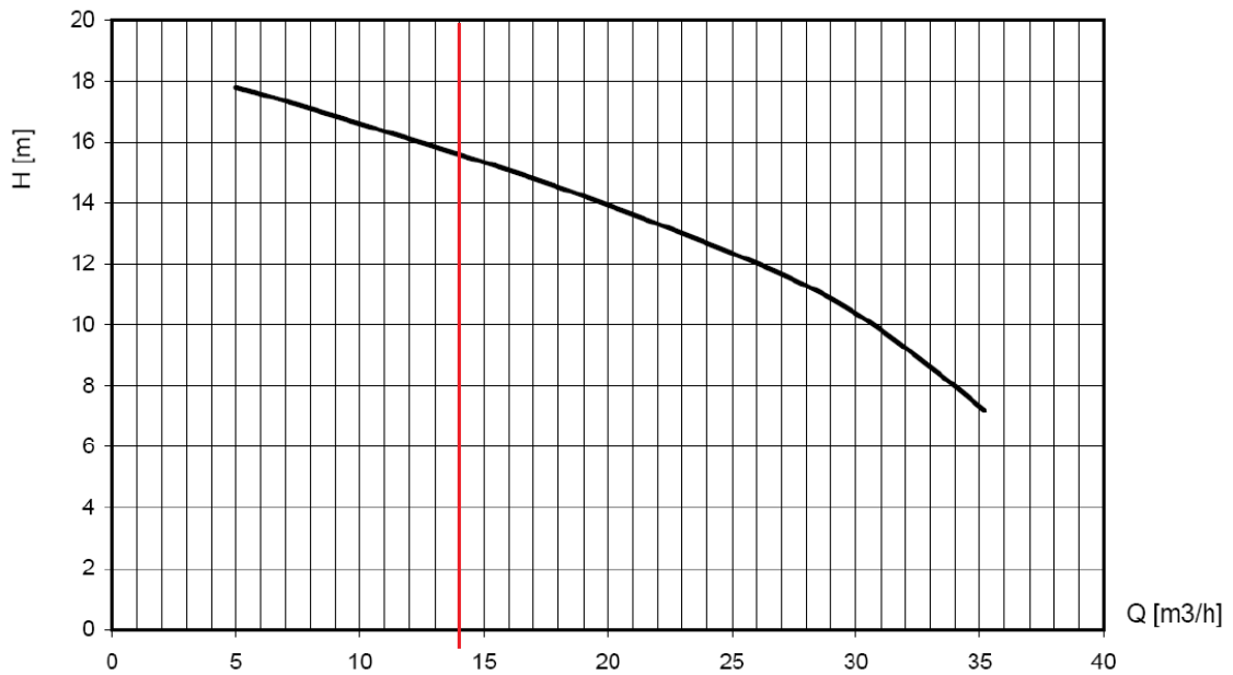
Figure 7.3: Total Head at different flows for B50 pump
