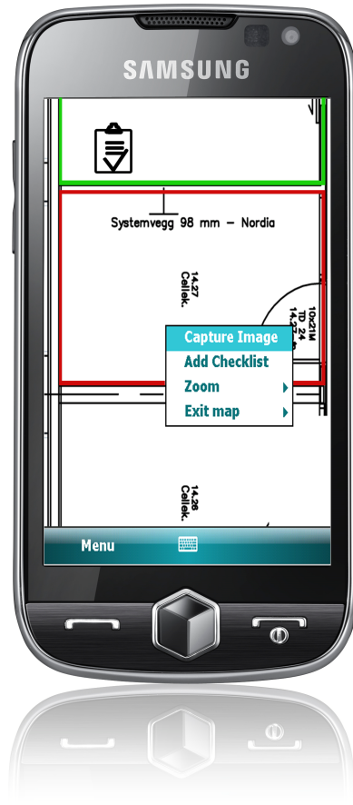
Figure 5.5: The cell phone application showing a construction site blueprint where a project manager has marked some rooms in the blueprint. The green room has been marked as finished, while there is still work left on the red room.
