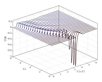
FIG. 3. (Color online) The TMR of an eight-junction array as a function of voltage and the product  $N\lambda$ . The parameters used are P = 0.3,  $\tau = 9 \times 10^3 R_0 C$ ,  $[N_0\Omega]^{-1} = 10^{-3} e^2/C$ , and  $k_{\rm B}T = 2 \times 10^{-3} e^2/C$ .
