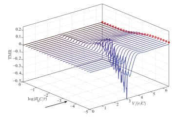
FIG. 4. (Color online) The TMR of an eight-junction array as a function of voltage and spin-relaxation time. The arrow indicates the time between tunneling events close to the threshold voltage (e/I @ 1.05 ×  $V_t$ ). The circular symbols shows the large voltage TMR from Eq. (8). The parameters used are P = 0.3,  $C_0/C = 2.5 \times 10^{-3}$  ( $\lambda \approx 0.05$ ),  $[N_0\Omega]^{-1} = 10^{-3} e^2/C$ , and  $k_BT = 2 \times 10^{-3} e^2/C$ .
