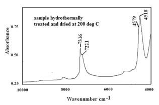
Fig. 2. Near infrared spectrum of hydrothermally treated silica gel sample
