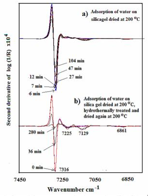
Fig. 5. Near infared spectra acquired in the region 7450-67500 cm<sup>4</sup> during the adsorption evolution of watermolecules
