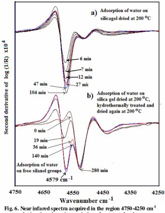
during the adsorption evolution of watermolecules
