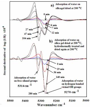
Fig. 3. Near infared spectra acquired in the region 5500-5000 cm<sup>4</sup> during the adsorption evolution of water molecules
