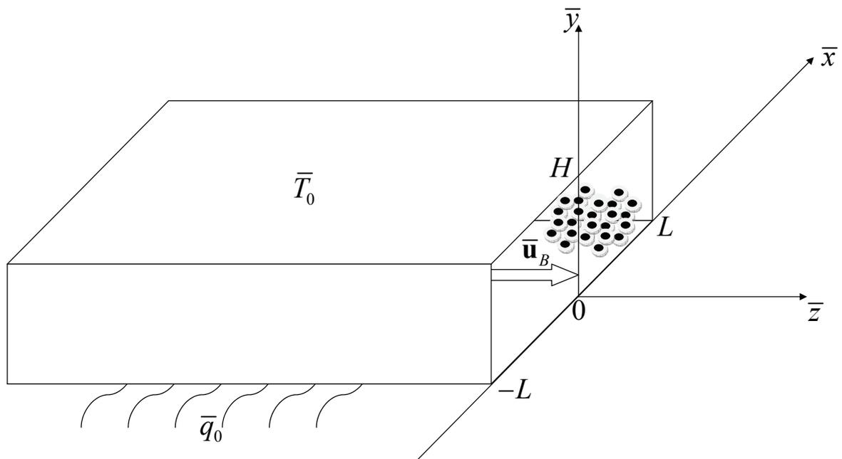
Figure 1: Drawing of the porous channel.
