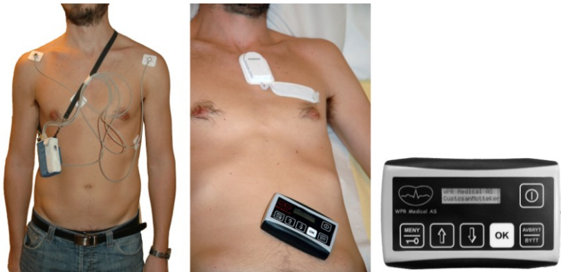
Figure 1. A picture of the Holter recorder with the cabled connections to the electrodes as used in the clinical trials (to the left), and the wireless ECG sensor placed on the chest (in the middle). A close-up photo of the hand-held receiver is shown to the right (different picture scales are used).
