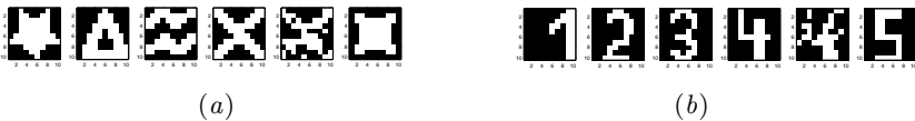
Fig. 8. The 10 \times 10 patterns used by Adachi et al (on the top) and Calitoiu et al (at the bottom). In both figures (a) and (b), the first four patterns are used to train the network. The fifth patterns are obtained from the corresponding fourth patterns by including 15% noise in (a) and (b) respectively. In each case, the sixth patterns are the untrained patterns.
