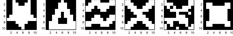
Fig. 2. The 10 \times 10 patterns used by Adachi et al. . The first four patterns are used to train the network. The fifth pattern is obtained from the fourth pattern by including 15% noise. The sixth pattern is the untrained pattern.
