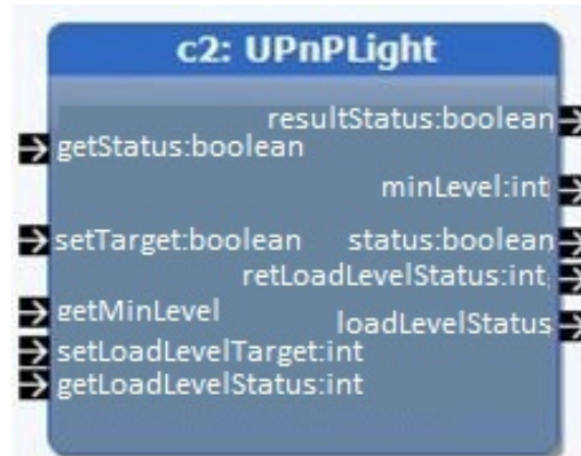
Figure 4.7: An ARCTIS building block is used to visually represent the UPnP Light service
