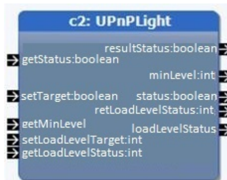
Figure C.1: An ARCTIS building block is used to represent run-time UPnP Light services, see also Figure 4.7
