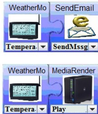
Figure E.3: The models of the new application defined in the scenario. Two puzzle compositions specify the structure and the behavior of the application.
