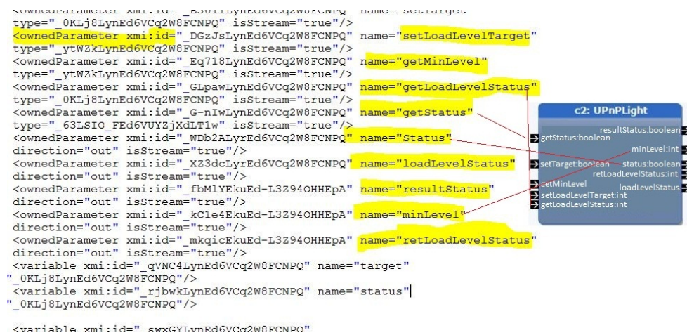
Figure 5.5: XML representation of the UPnP Light service in an ARCTIS building block presented in Figure 4.7. The XML contains information about operation names, xmi:id, arguments, type of arguments, directions, etc.
