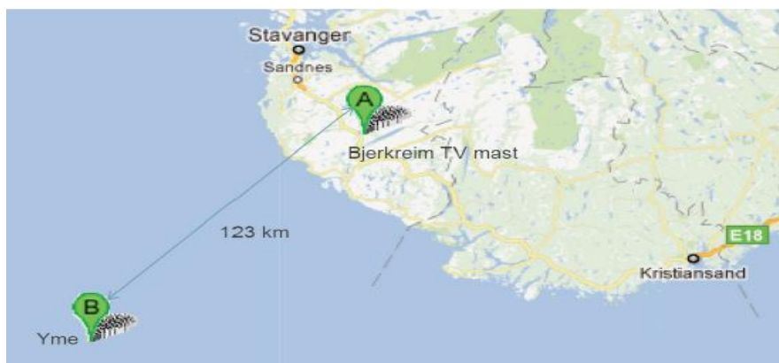
Figure 2-4 Ceragon 123km over-water link [10]
