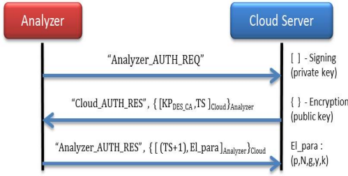
Fig. 2. Mutual Authentication between Cloud server & Analyzer
