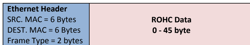
Figure 4.3: Ethernet frame for the 0x8889 protocol type [21]
