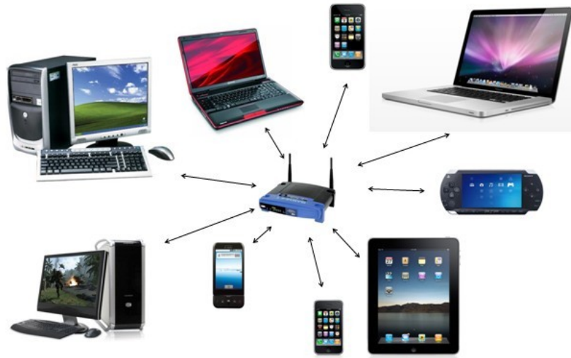
Figure 1.1: Home local area network with a router
