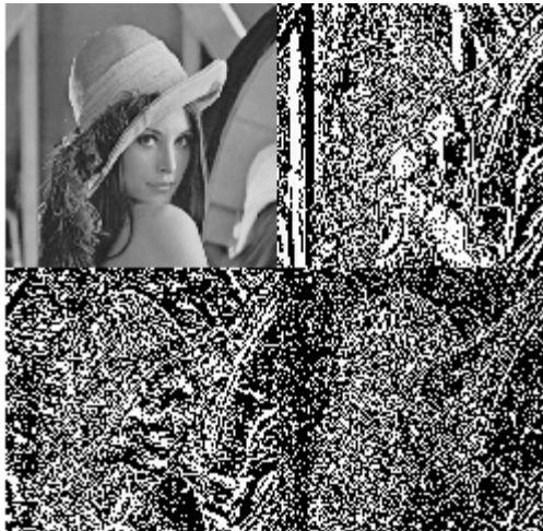
Figure 4.15 (b) A single pass of the transform, showing the three sets of coefficients, and the residual filtered image. [7, 15]
