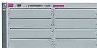
Figure 40 HP Procurve 5300 Series Switches - Layer 2, 3 and 4
