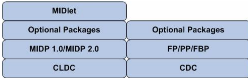
Figure 2.7 An illustration of the MIDlet on top of the MIDP/CLDC structure
