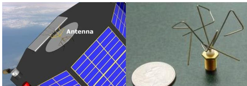
Figure 15 Satellite antenna designed by GA [9]
