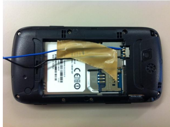
Figure 5.2: power measurement performed in Lab 2
