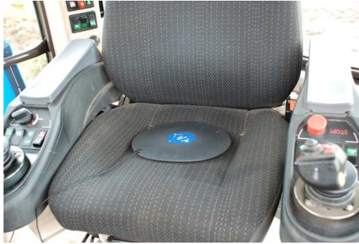
Figure 4: SV 39A Whole-Body Seat Accelerometer placed on seat.
