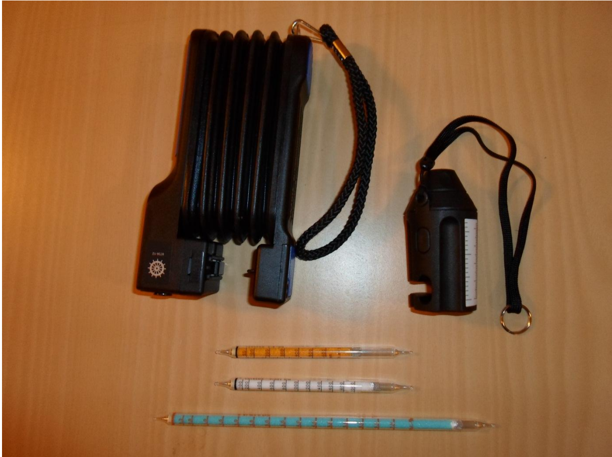
Figure 4.2 Dräger Tubes, pump accuro and tube-glass breaker
