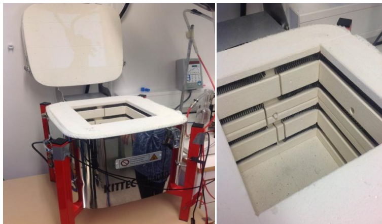
Figure 4.3: The furnace and the burning coils inside the furnace
