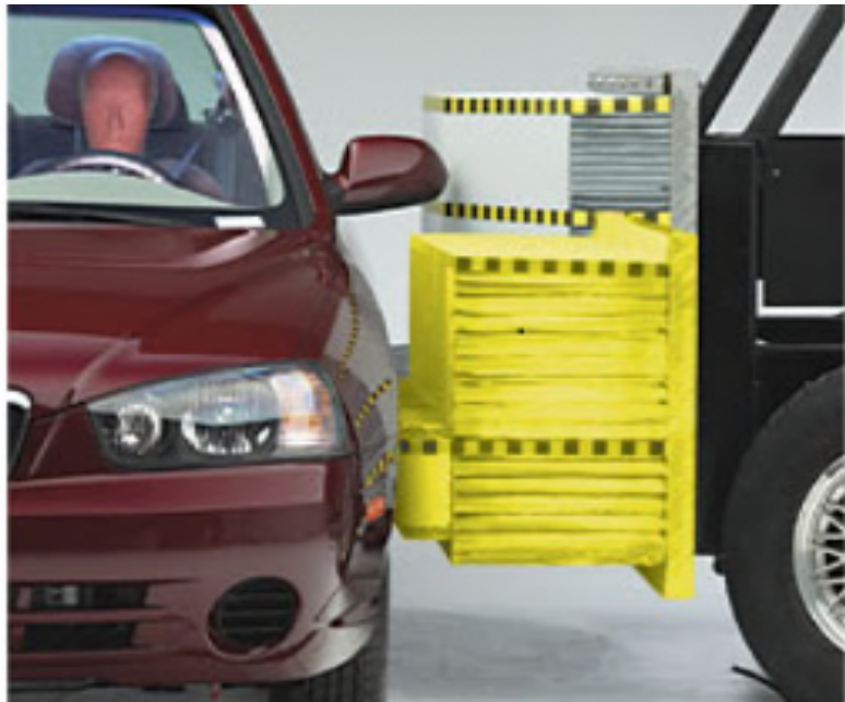
FIGURE 2.7: IIHS Side Impact Test Set-Up [3].
