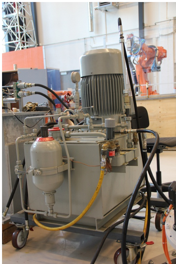
Figure 7.1: Transportable Hydraulic Power Unit
