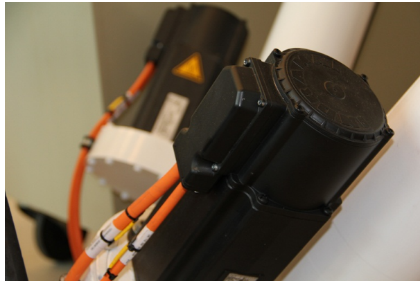
Figure 2.4: Power and Signal Cable to each Servo Motor
