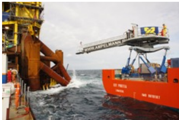
Figure 1.1: Ampelmann's Heave Compensated Walkway [2]
