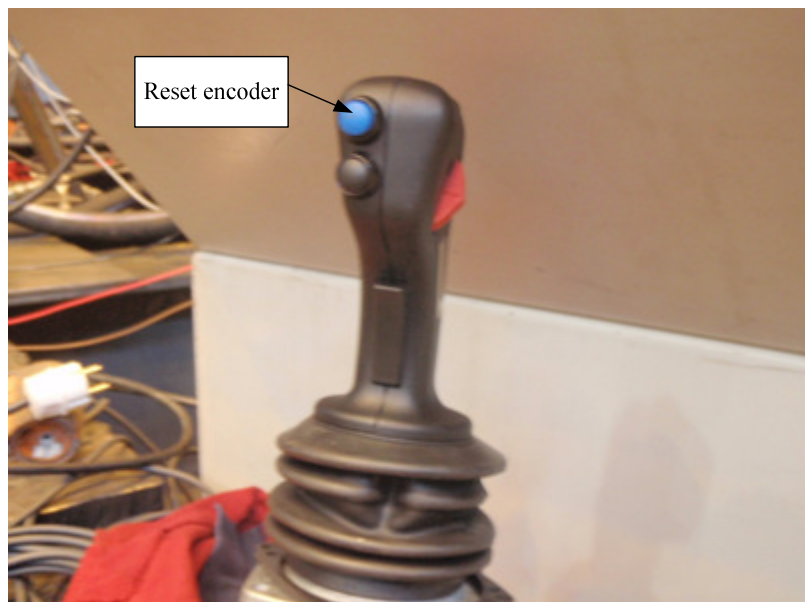
Fig 5.18 Button used for reset the encoder
