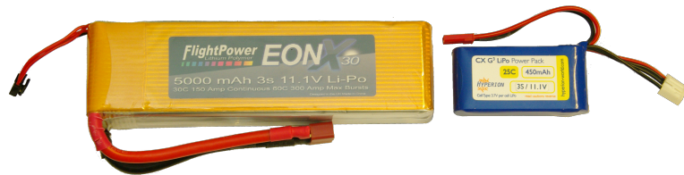
Figure 4.14: Batteries used, to the right 5000 mAh and to the left 450 mAh
